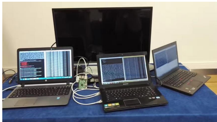
Fig. 1. A private Ethereum Blockchain running in a local network area (LNA) used for distributed energy trading
